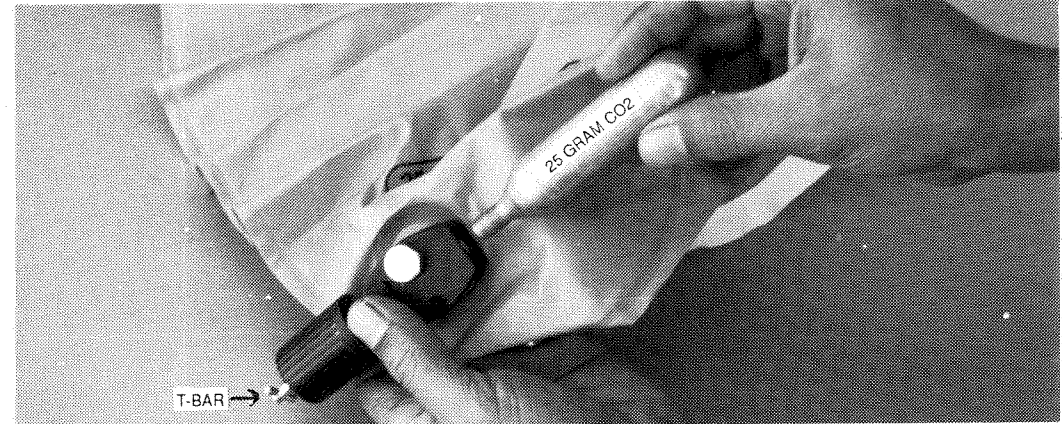
7. Install new 25 gr. CO2 cylinder. Hand-tighten only.
