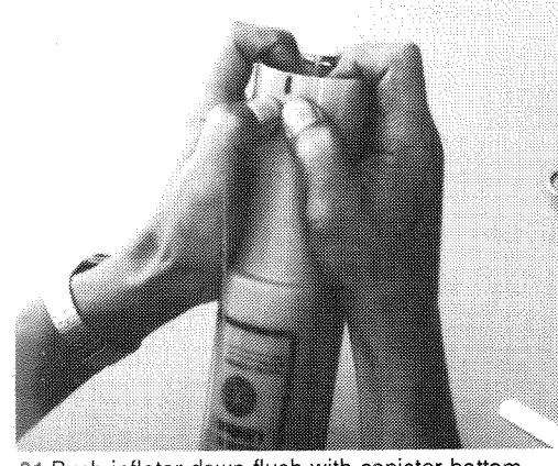
21. Push inflator down flush with canister bottom.
